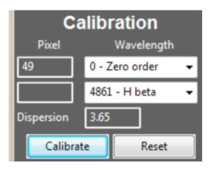
You can undo the calibration and start over by pressing the **Reset** button. Also, if you didn't click exactly on the right spot when adding your calibration points and your calibrated curve isn't matching your reference lines (see below) perfectly, you can tweak the calibration by editing the pixel values in **The Calibration Area** and then press
