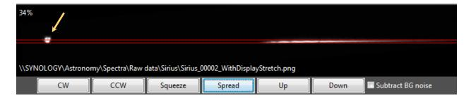
Once you get the spectrum centered and zoomed appropriately, you can rotate it clockwise or counter clockwise as needed by pressing the **CW** and **CCW** buttons, respectively. The image will rotate 1 degree or 10 degrees if you hold the **Shift** key when pressing the buttons.
