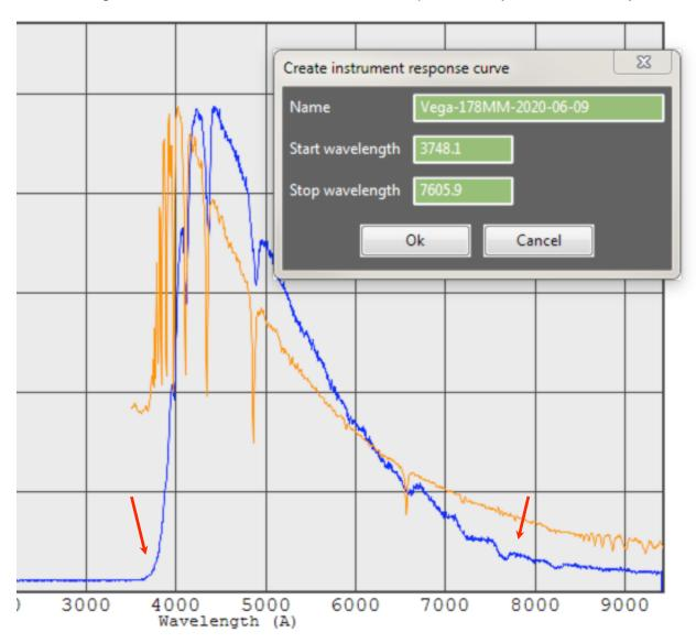
not have the same sensitivity to a wide range of wavelengths as the reference. So we want to limit it in order to make a useful IR curve. Basically, only include areas on the curve that show a meaningful response above the baseline. The example shows two red arrows that specify a start and stop wavelength. Right click on a spot and choose **Set start/stop wavelength for IR response curve** from the popup menu. Do this twice,
