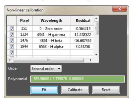
Once you have your pixel wavelengths defined, choose an order from the **Order** list and press **Fit**. A polynomial will be generated to fit the data and the errors for each point will be displayed in the **Residual** column. The actual coefficients of the polynomial will be displayed as well. Press the **Calibrate** button and display some reference lines on the spectrum to see how well the fit is.
